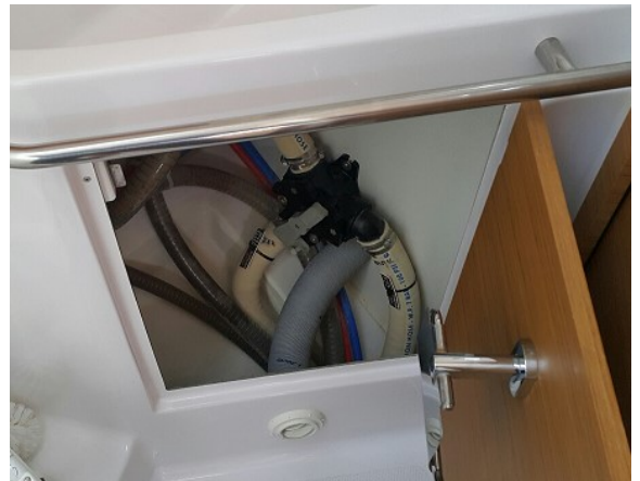
Handle to switch between waste tank and sea
