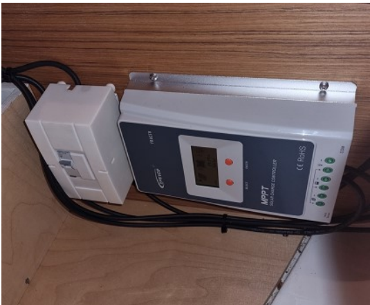
Solar panel switch and charger located under the bed of starboard aft cabin
