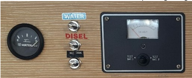
Switch on for level indication of fresh water, waste tank or diesel tank.
