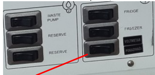
Switch on for level indication of fresh water, waste tank or diesel tank.
