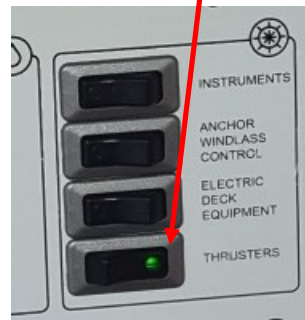
Remote control of bowthruster Quick (maximum time of continuous operation 5 seconds to avoid overloading)
