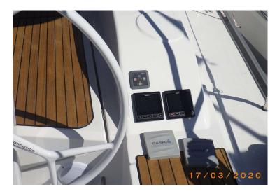
Charter plotter Garmin GPSMAP 742 and **ship's compass** located at the cockpit table.
