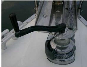
Remove the safety line and push the anchor over the bow, keeping hands and feet clear. Control the rate the chain pays out by tightening or loosening the brake with the windlass handle.
