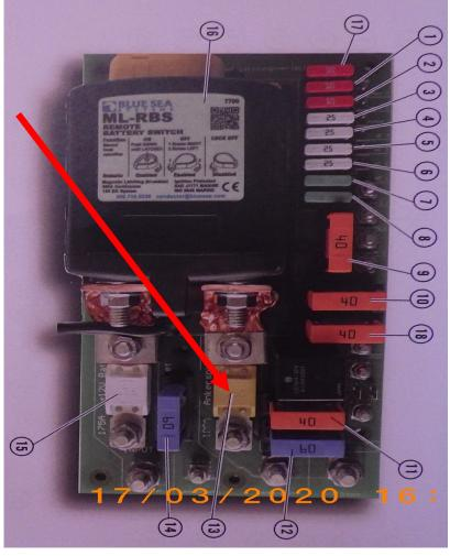
If the windlass is not workable, but the windlass breaker on the 12v panel is switched on, and that the green light is illuminated, this indicates that the yacht service battery power is too low to run the windlass. Please run the engine @1500 rpm for 15 min, and try again. If the windlass still refuses to operate, please call technical support.
