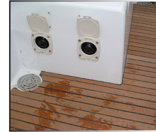
MANUAL BILGE PUMPS
