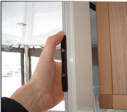
OPENING SERVING HATCH BLOCKING SYSTEM
